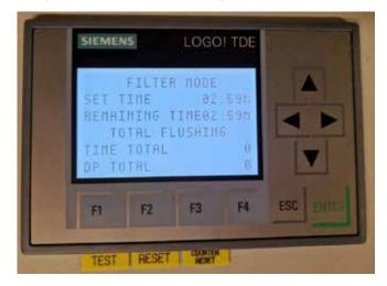
Find "LOGO! SETTINGS" line by using "UP and DOWN ARROWS", and press "ENTER", Find "PROGRMAN" and find "SET PARAMETER" line by using "UP and DOWN ARROWS", and press "ENTER", Find "FLT TIME" line by using "UP and DOWN ARROWS", and press "ENTER"
