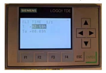
In options, the [T =] means the set time for given parameter. The [Ta =] means how much time has passed towards the set T
